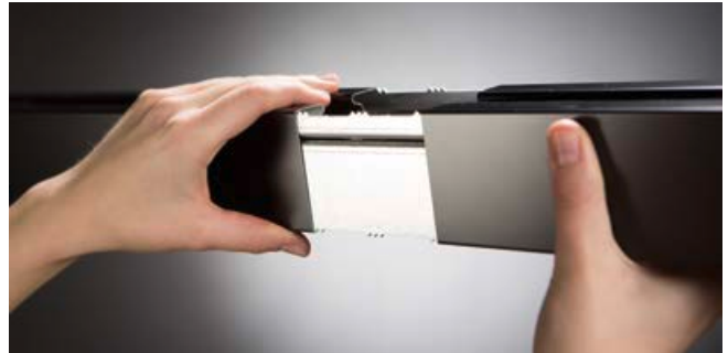
The individual carrier rail segments are joined with longitudinal connectors and secured with screws.
